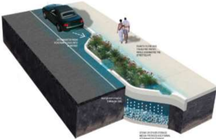
Mid-block Stormwater Bump-out
