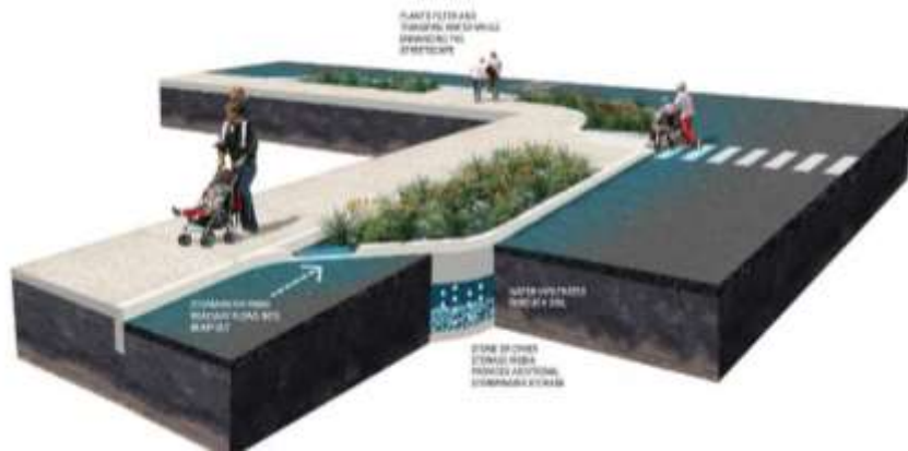
Corner Stormwater Bump-out
