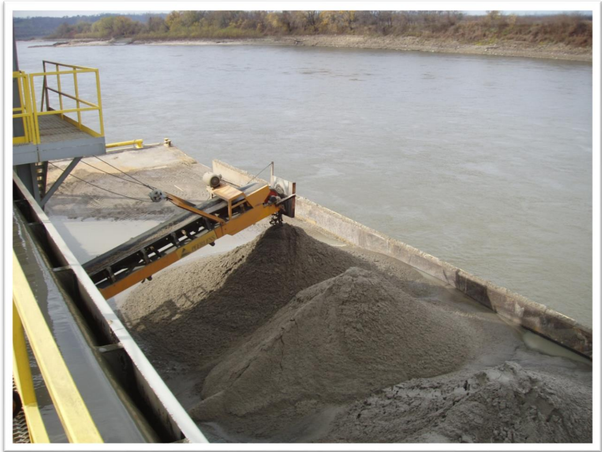
Figure 4-1: A commercial sand and gravel mining operation. Material is mined from the riverbed using a hydraulic dredge.
