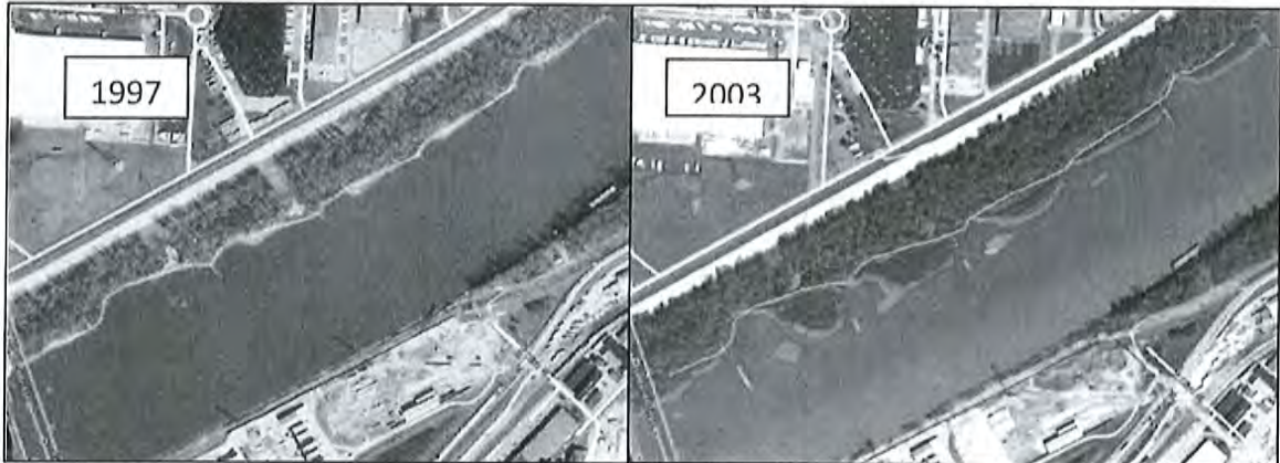
Figure 2: Example of accretion and vegetation (river mile 364) caused by perched structures.
